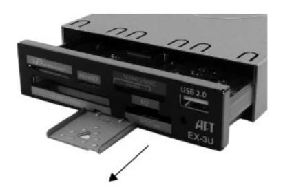
Push SERVICE KEY into slot until you feel it has locked onto the Bezel/PCB.
