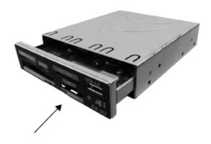
Once NEW Bezel/PCB is installed into EX-3U Chassis, you can power up your system and test the NEW Bezel/PCB.
