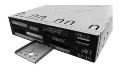
Insert SERVICE KEY into key slot located under the CF and MS card slot.
