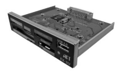
After removing the OLD Bezel/PCB, take NEW Bezel/PCB and insert into housing of EX-3U.
